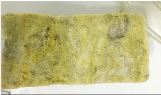
Figure 2. Dark mould fungi on the surface of rockwool.
