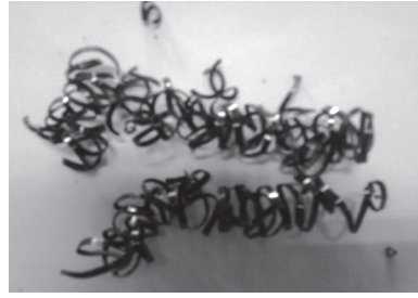
V_c = 46 \text{ m/dk}, f = 0.22 \text{ mm/dev}
